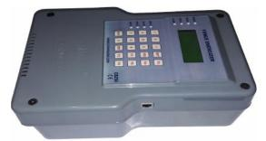
Parameters like Fence voltage, SPV voltage, Battery voltage, Mains status and settings for Alarms can be viewed using **Front Panel Keypad and LCD** OR **from Web Browser using In-built Web server**.
